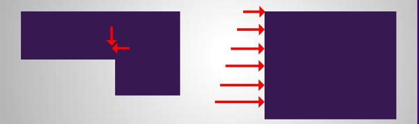
ASCE7-05 requires that accidental torsion be considered for both orthogonal directions, and orthogonal interaction effects are permitted to be neglected base on the seismic category B. Forces along with moments due to torsion were applied at each story level in order to transfer the load through the diaphragm to lateral elements.
