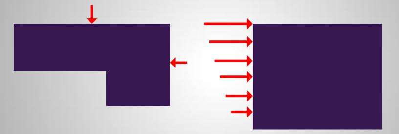
ASCE7-05 requires four different wind loading conditions be applied in order to account for quartering winds and torsion. Pressures were calculated for these four cases and applied as forces each story level using tributary area in order to transfer the load through the diaphragm to lateral elements.
